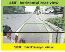
A 2-in-1 image of the horizontal rear view and the bird's-eye view display in LCD monitor
